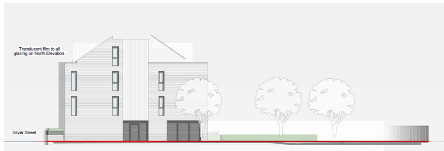
⑥ Elevation 6 - North 1:100
